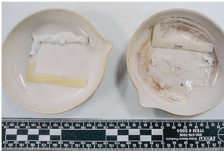
Nylon parts before and after ash tests. Good part on left, bad part on right.
