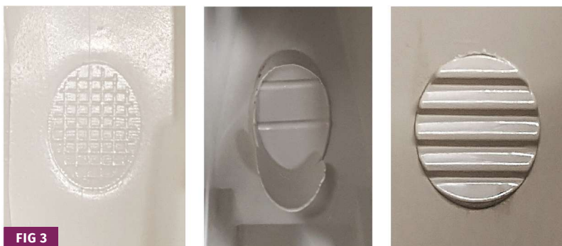
(L. to R.) Cross-hatched, partial and full stair-stepped ejector-pin faces. Notice the down-flash primarily on one side of the partial stepped pin.
