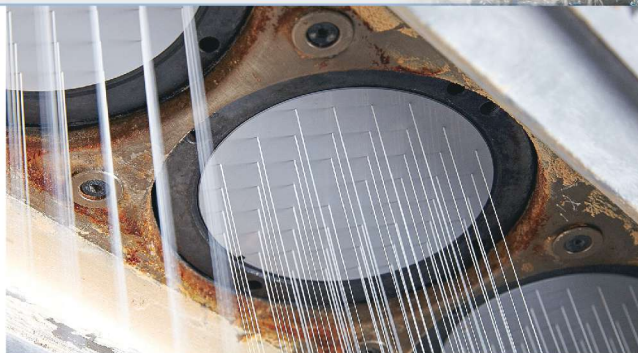
In the Repreve recycling process, pellets (or "chips") are melted and extruded into a fiber.
