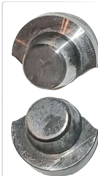
Differential temperatures can even cause interlocks to break.
