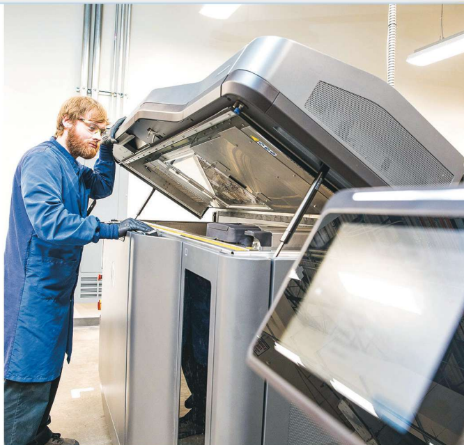
Protolabs has a 77,000-ft 2 plant devoted to five different 3D printing technologies using thermoset, thermoplastic, and metal materials. Its newest technology, shown here, is HP’s Multi Jet Fusion, which is said to be 10 times faster than other 3D-printing processes and to produce parts with properties closer to those of injection molding.
