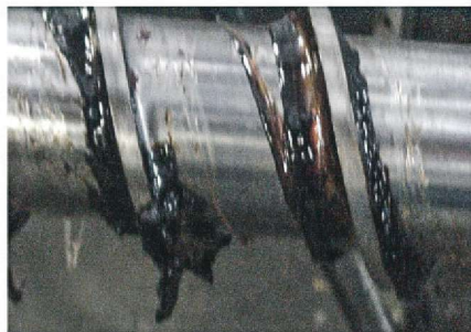
Clear resin shows significant degradation as a result of getting hung up on a dead spot in the screw for too long.
