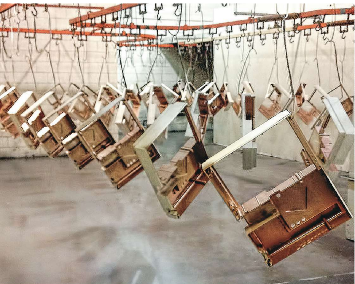
Spray-on shielding reduces the number of parts used on instruments, eliminating the cost of a box within a box and associated attachment parts.
