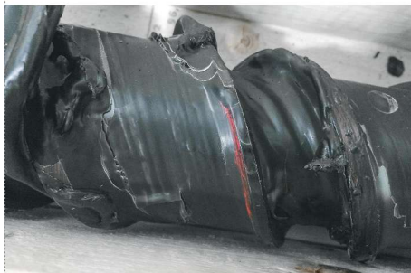
FIG 2 Red Material 'Hangup' On Flights
