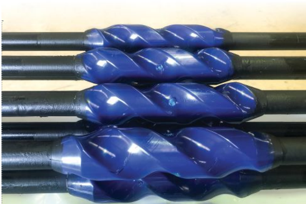
Synthetic Metal concept is used to create sucker rods for the oil and gas industry.
