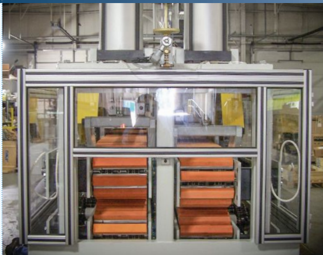
Dual cleated pullers manage separate line speeds to maintain proper quality for each profile.
