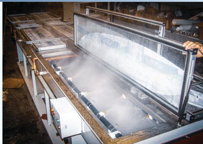
Dual-sided spray tanks provide high-intensity evaporative spray cooling for larger profile extrusions or for profiles made of wood-plastic composites or other materials that have high cooling requirements.
