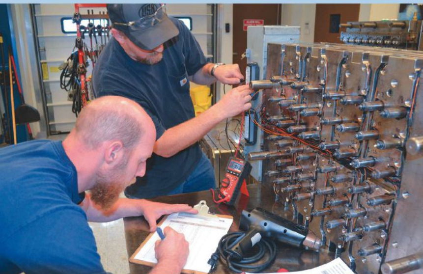
After the ohm reading is concluded, matching ohms to the pin number on the connector, use a heat gun to verify that the positions match the pin numbers.
