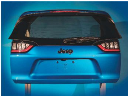
The body exterior winner was the thermoplastic liftgate that replaced a steel design on the 2019 Fiat Chrysler Jeep Cherokee SUV.
