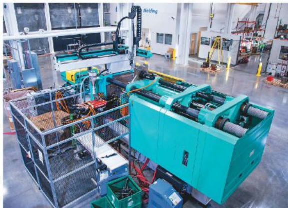
Core Technology's second two-shot molding cell was built around an E-Multi secondary injection unit and an Arburg injection molding machine.
