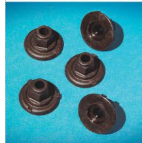
This high-strength, self-tapping composite nut of 55% glass-filled nylon 66 on the 2016 Fiat Chrysler Pacifica minivan won the chassis/hardware category.
