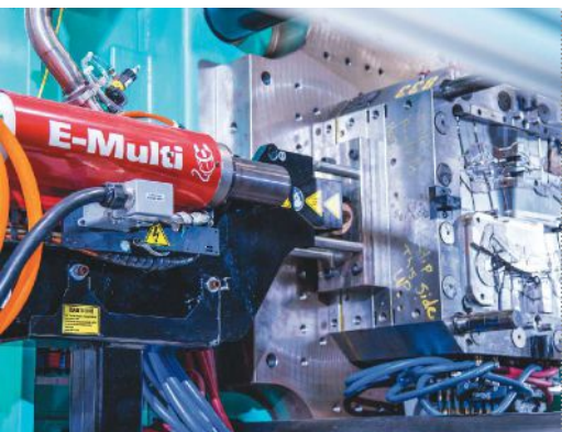
The second of Core Technology's two E-Multi auxiliary injection units features a 24-g shot size.
