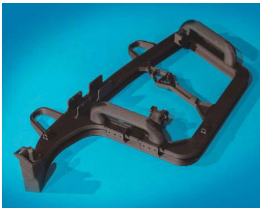
The window-alignment fixture in the 2017 Ford Mustang was produced by Stratasys using its FDM additive manufacturing process and nylon 12 with 35% short carbon fiber.
