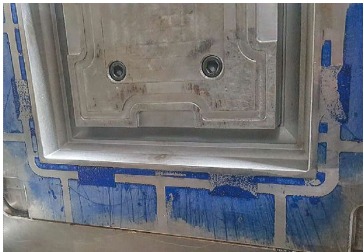
Bluing off a mold is a good way to check the condition of the vents.
