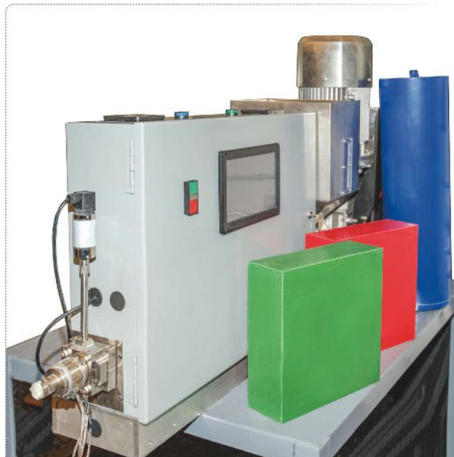
Extruder section of Omachron molding machine, with molded parts, including an 8-in.-diam. HDPE rod (blue).
