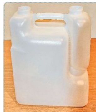
Another EBM challenge in HDPE: This two-chamber part with a blown neck.
