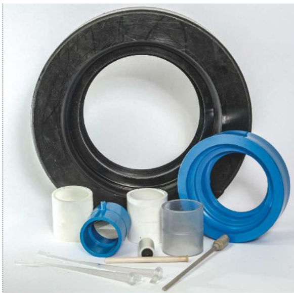
More thick-walled parts molded on Omachron low-pressure injection machine.
