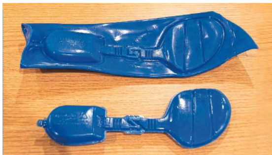
The TPU Reebok Dynamic Mid-Sole was the job that got MSA into production molding for technically challenging jobs.
