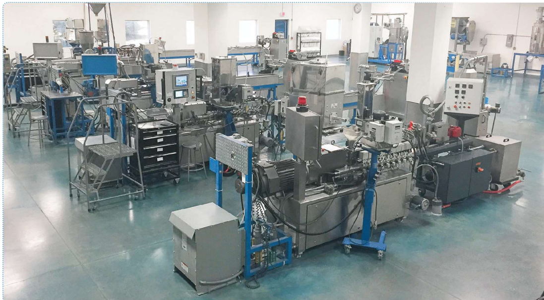
Compounding Solutions' white room is equipped with a HEPA-filtered air exchange with humidity and temperature controls, and epoxy-coated wall surfaces to repel dust and allow for easy cleaning of all surfaces.
