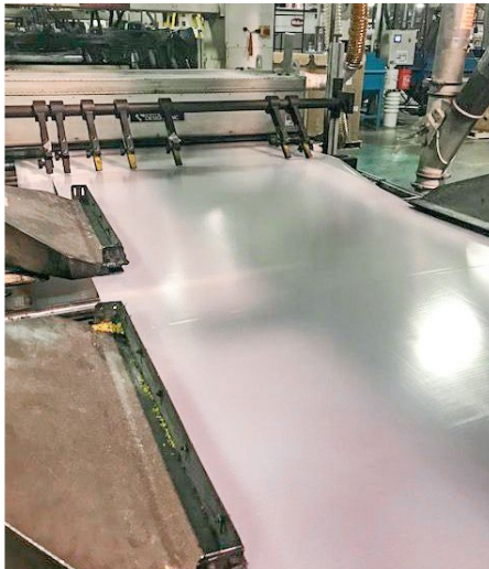
MDI runs two coextrusion lines for corrugated HDPE sheet in Grand Rapids, and is looking to add a third line for PP.
