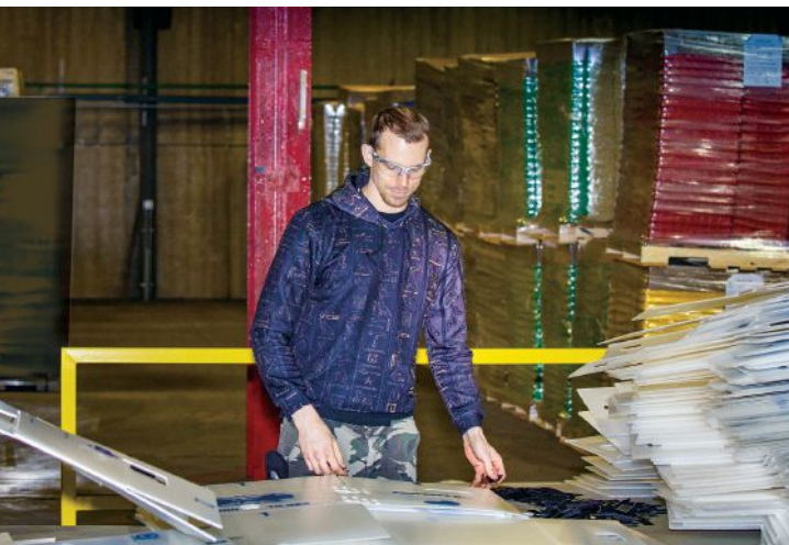
MDI is vertically integrated in corrugated HDPE tote manufacturing. Extruded sheet is die-cut, printed, folded and ultrasonic welded in house.
