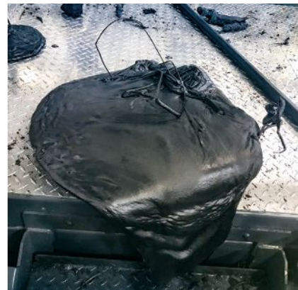
Purge should be removed from press bed to prevent sticking. Keep your press bed and area clean and free of debris. Best practice is to treat every day as if the customer will walk the floor at any minute.
