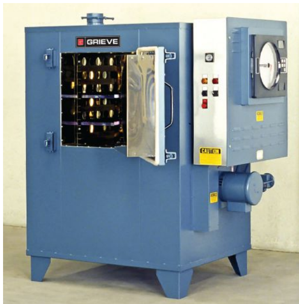
The target annealing temperature is often the midpoint between T_g and T_m . Lower temperatures will require a longer annealing time. (Photo: Annealing oven from Grieve Corp.)
