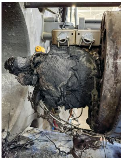
Failing to pull back the carriage at shutdown can lead to blowback when the press is restarted.
