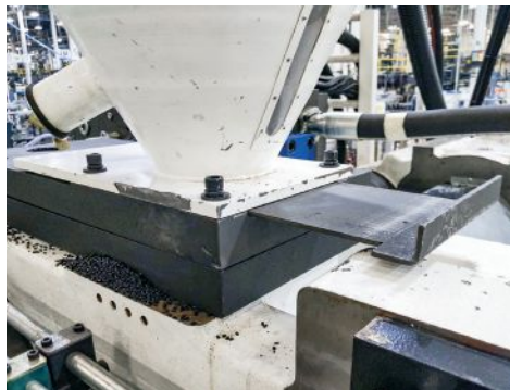
Failing to close the slide on shutdown can lead to a bridged throat and excessive downtime.
