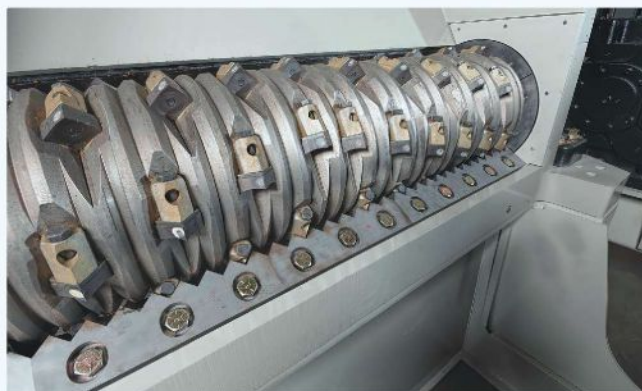
To reduce frictional heat and improve shredder performance on very tough purgings, the solution may be a water-cooled rotor and a boost in horsepower.
