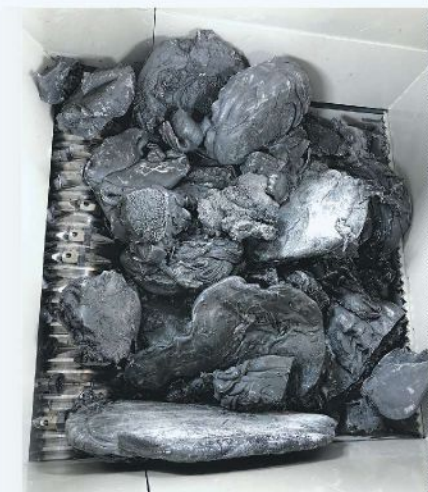
Shredding heavy, dense purging scrap can be a challenge, depending on the formulation of the purge material.
