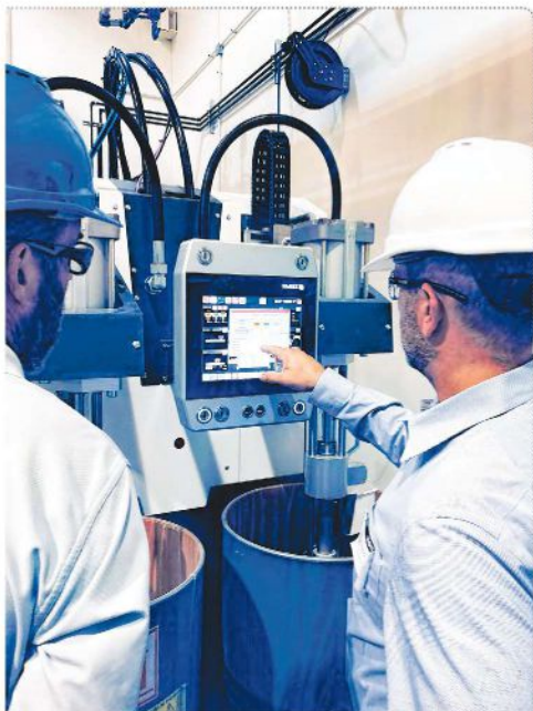
Ability to "dial in" cure time, temperature, and Shore hardness offers new flexibility to LSR molders. (Photo: Elmet)
