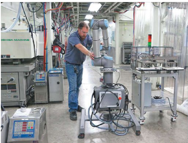
Cobots can easily be moved from press to press, as seen here at Dynamic Group.
