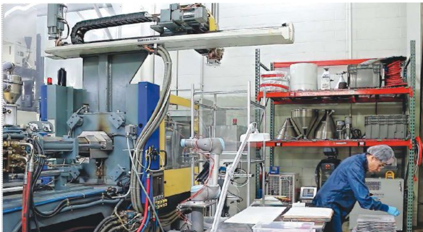
At 2D&S in the Czech Republic, a UR10 inserts IML foils into the injection mold.
