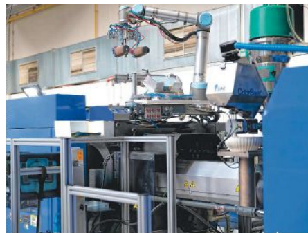
At 2D&S in the Czech Republic, a UR10 inserts IML foils into the injection mold.
