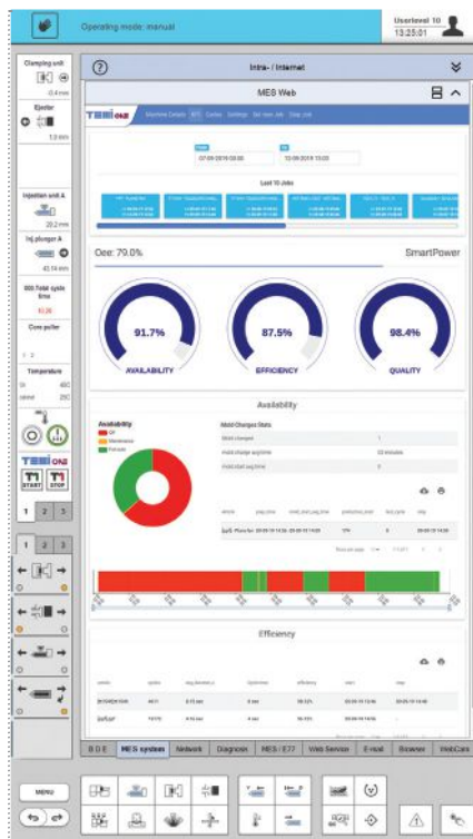
TEMIone is a new MES for a single injection machine, integrated into Wittmann Battenfeld’s B8 controller.
