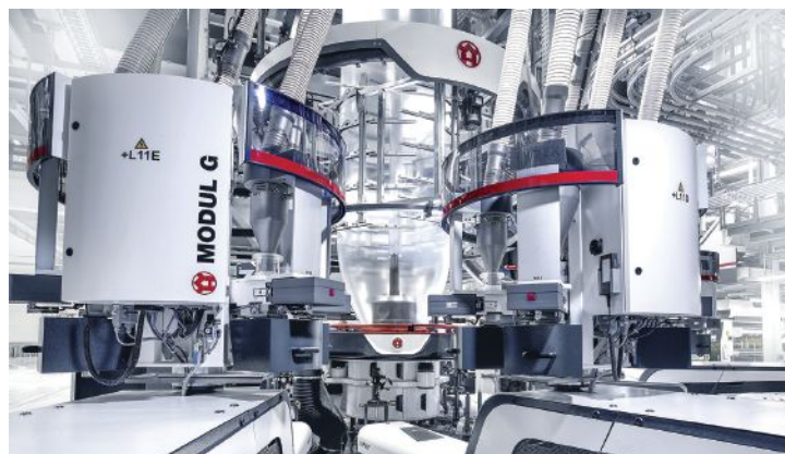
During the K 2019 show, W&H demonstrated its Turbostart automation system on a Varex II line, stopping and restarting a blown film line 50% faster, safer, and easier.
