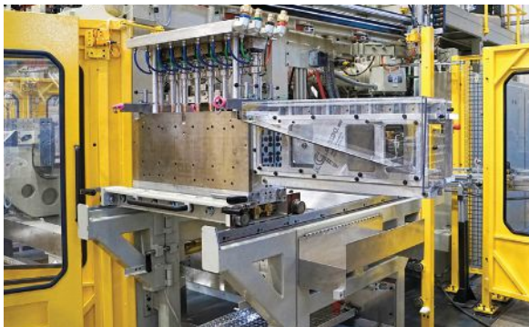
Bekum's new Concept 808 shuttle machine debuted with optional magnetic quick mold clamping—possibly a first in blow molding—which allows changeover of molds and blow pins in 15 min per side.
