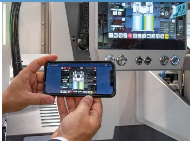
Elmet showed its new servo-driven TOP5000E LSR dosing system with web connectivity and remote monitoring/control via mobile devices.
