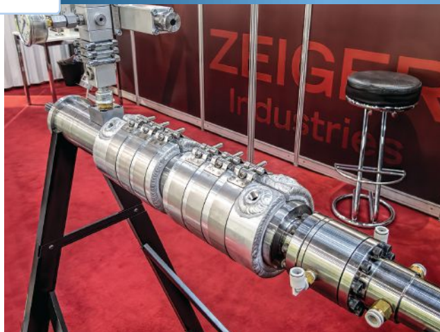
Zeiger Industries' latest LSR conversion packaging includes quick-disconnect water jackets and a pump connection without threads that can lock up if exposed to resin leaks.
