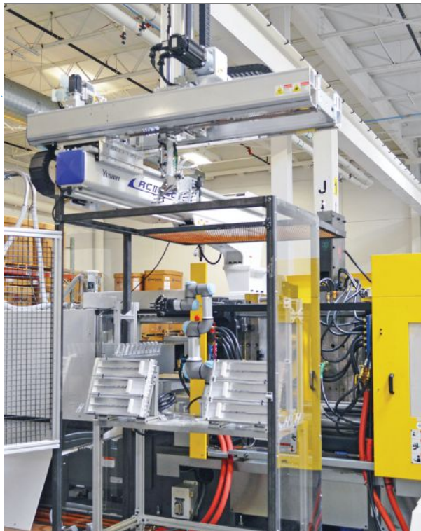
Tenere has embraced automation as a means to boost productivity, pairing a traditional three-axis Yushin robot with a UR cobot in this cell.
