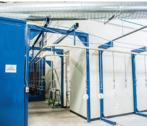
An automated paint booth supports Tenere's enclosure business, including painted bezels.
