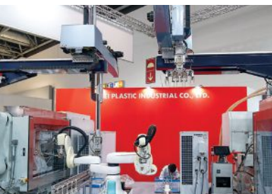
Nissei molded PLA champagne flutes in two parts on two presses. Two top-entry robots (left) delivered the parts to a Kawasaki dual-arm DuAro SCARA-type cobot that assembled the flutes (right).
