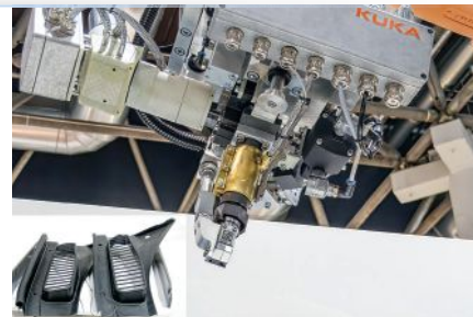
Kuka introduced a new extrusion head for its six-axis robots, which can deposit gaskets directly onto molded parts (inset, left).
