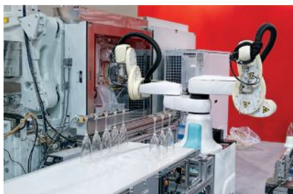
Nissei molded PLA champagne flutes in two parts on two presses. Two top-entry robots (left) delivered the parts to a Kawasaki dual-arm DuAro SCARA-type cobot that assembled the flutes (right).
