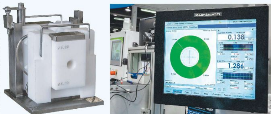
FIG 4 Extruded tubing passes through an immersed ultrasonic gauge, which reads its wall thickness and displays real-time output on a screen. (Photos: Zumbach Electronics)
