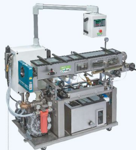
FIG 3 Controlling the size of small-diameter, single- or multi-lumen medical tubing has required machine builders to scale down the size of previous vacuum-sizing machinery to provide greater process control.
