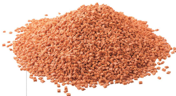
A new grade of Ixef semi-aromatic nylon is colored “signal orange” for use in electric-vehicle rechargers. Despite 50% glass content, it reportedly offers high flow in thin sections and a glossy, resin-rich surface.
