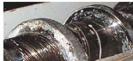
The solid break-up that can occur when processing semi-crystalline materials leads to some partially unmelted pellets getting through the transition and metering zones of the screw. These partially unmelted pellets can wind up in the part (left) and wear the screw (above), even this one running only PE.
