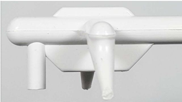
If an ejector pin is too far away from a tunnel gate, adding stiffening ribs to the runner will reduce its flexibility.
