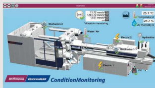
Condition Monitoring System Predictive Maintenance
