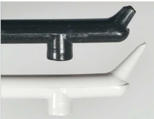
Determining the location of the ejector pin that forms a boss for a tunnel-gated mold that will run multiple materials is especially challenging.
