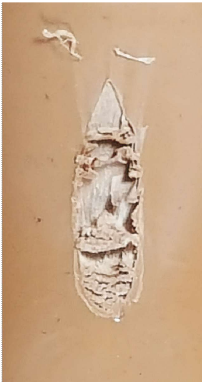
An ugly tunnel-gate scar is often caused by more than just one problem.
