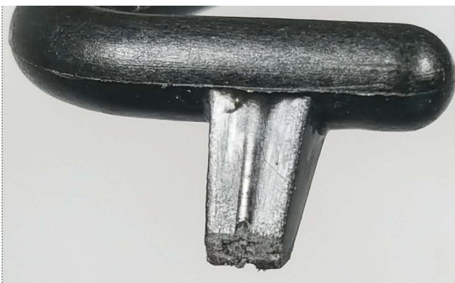
Converting elliptical gates to chisel gates often solves a flaking problem.
