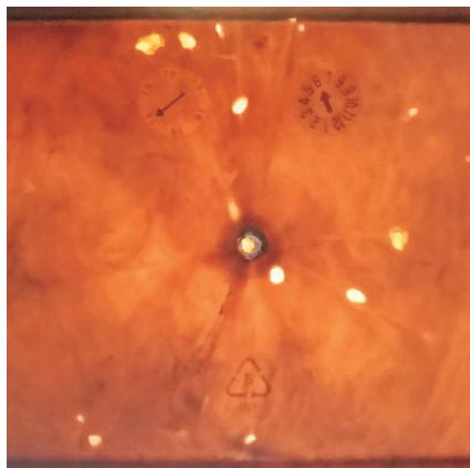
The solid break-up that can occur when processing semi-crystalline materials leads to some partially unmelted pellets getting through the transition and metering zones of the screw. These partially unmelted pellets can wind up in the part (left) and wear the screw (above), even this one running only PE.
