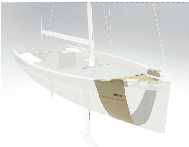
Two new Thermocomp AM compounds were used for a concept boat hull from Livrea Yacht—a carbon-fiber reinforced PEI for the inner lattice support structure.
