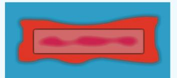
When a plastic strand enters the water bath, it heats the water around it or forms a steam jacket. As a result, the water bath is trying to cool that hot water layer before it can cool the strand. This delays the cooling effect of the water bath. In the absence of any turbulence, you're basically left with trying to cool hot plastic strands with warm water a sub-optimal cooling situation. (Photo: Conair)
