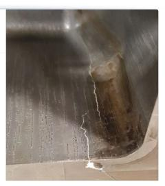
A cavity insert cracked at an inside corner.
