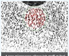
A new microscope allows lab staff at Teel Analytical Laboratories to determine foam cell formations so they can optimally tweak their extrusion process
