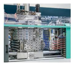
With the two materials injected into mold faces 180° apart, the only way to provide two cooling stations for each, and to eject on the same side of the machine, was to split the mold into sections rotating in opposite directions. In the fourth mold station (on the non-operator side of the machine), a six-axis robot demolded the parts while assembling them with a snap fit. In this way, the same cavities and components are always
