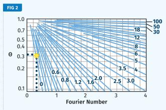
With the blue line numbered 0 and approach temperature, you can determine your Fourier number from the Heisler chart. You take your approach temperature  $\Theta^*$  on the left and go to the right until you hit the line that represents your inverse Biot number. As shown here, the Fourier number is around 0.32.
