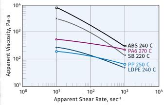
The shear-thinning effect is different for every polymer and grade. The individual curves are also offset up or down as the temperature decreases or increases, respectively. How the shear rate and temperatures affect polymer viscosity in the tooling can result in considerable variations in pressure drop through the die.
