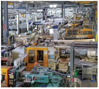
TG Missouri is gradually converting over 100 hydraulic presses to a high-performance hydraulic oil—Mobil DTE 10 Excel 46—that saves energy, better protects valves, and keeps the system cleaner.
