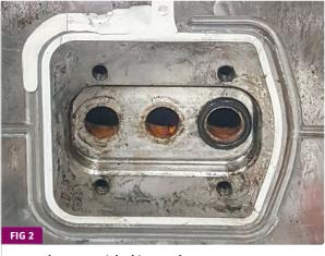
A core insert stuck inside a cavity.
