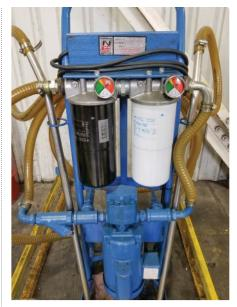
Data-based maintenance management prompted other changes, such as using more efficient hydraulic filters.
