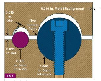
A cylindrical interlock protecting a cylindrical core pin.
