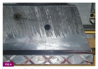
Wear on the side of a cam due to plate misalignment.
