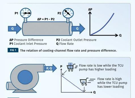
FIG 2 The inverse relationship between flow rate and pressure from the TCU pump.
