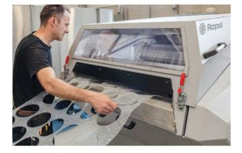
Running the new machine at the low end of the speed range helps improve regrind quality for highly brittle materials by minimizing dust generation, Rapid says. Reducing rotation speeds from 25 rpm to 15 rpm also reduces noise levels by as much as 3-5 dba. Running the machine at higher speeds improves cutting of soft materials and allows molders to increase capacity by 30-40%. The torque level of the machine is maintained regardless of the speed at which it is running.
