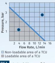
FIG 3 The loadable area of the TCU, as determined by simulation of the total flow and pressure requirements of all cooling channels.
