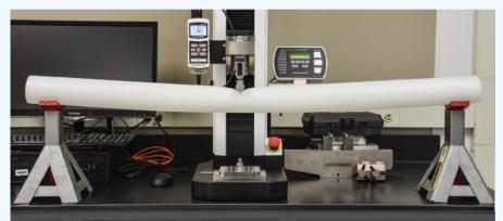
Extruded core testing for film winding has led the Teel lab team to work on different cooling techniques—particularly with polyolefin cores—to counteract the annealing that occurs on the ID of the core.
