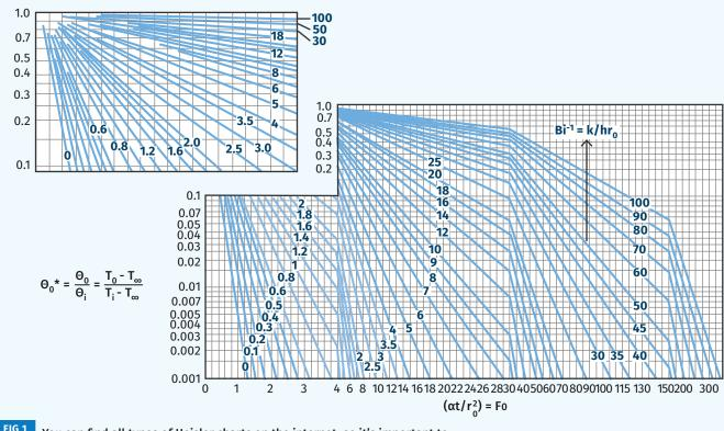
FIG 1 You can find all types of Heisler charts on the internet, so it's important to pick the right one for your calculations. This one can be used for strand pelletizing.
