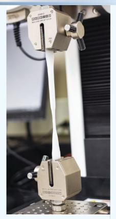
Final product testing at Teel includes mechanical analysis such as tensile strength, along with chemical and physical testing.
