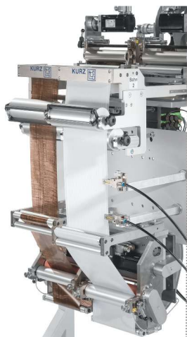
Kurz Duo SI IMD reel-to-reel system feeds two independent single-image foils through a two-cavity mold using servo drives, optical sensors and registration marks on the foils for precise positioning.
