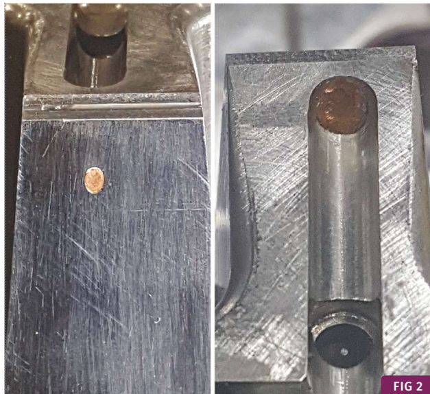
Shown here are subgates blocked with copper, which unfortunately is a common technique.
