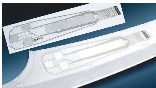
Kurz Functional Foil Bonding (FFB) uses its PolyTC sensors, with electrical circuits printed on a PET carrier and connected to an integral plug. These are applied after molding the part, using vertical or roll-on hot stamping. The flexible sensors conform to curved surfaces.
