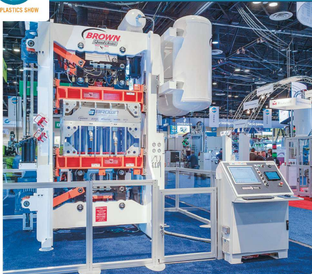
Brown Machine's new Quad Series thermoformer is available with a dual servo-drive system that maintains coining force at higher speeds.
