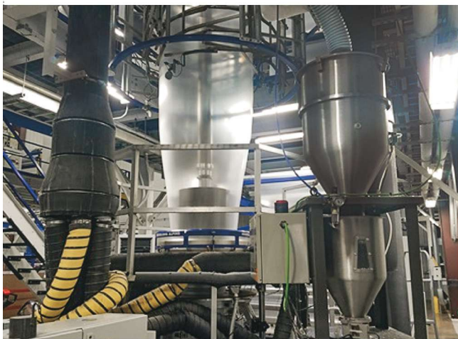
Berry runs three-layer coextruded blown collation shrink film made of various PE blends to achieve low haze, cuttability, shrinkability, and sealability.
