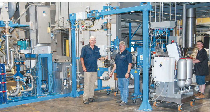
BPC Toll Compounding & Blending recently accepted delivery of ENTEK's high-output HR 3 73-mm, 48:1 L/D twin-screw extruder. Pictured (l-r) Mike Krause, general manager; Reggie Dunn, process manager; and Austin Castleberry, operator.
