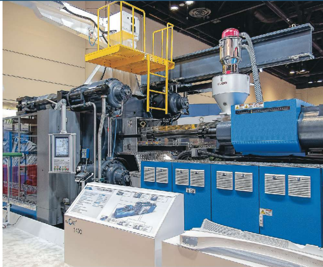
Lucky Goldstar (LG) is back, under the name LS Mtron. The One is its new premium line of servo-hydraulic two-platen presses.
