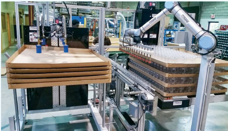
Proco Machinery has developed packaging systems for blow molding, like this Half Cube Palletizer, with Universal Robots cobot arms to reduce the handling of containers, simplify operation, and enhance efficiency with a small footprint and fast ROI.
