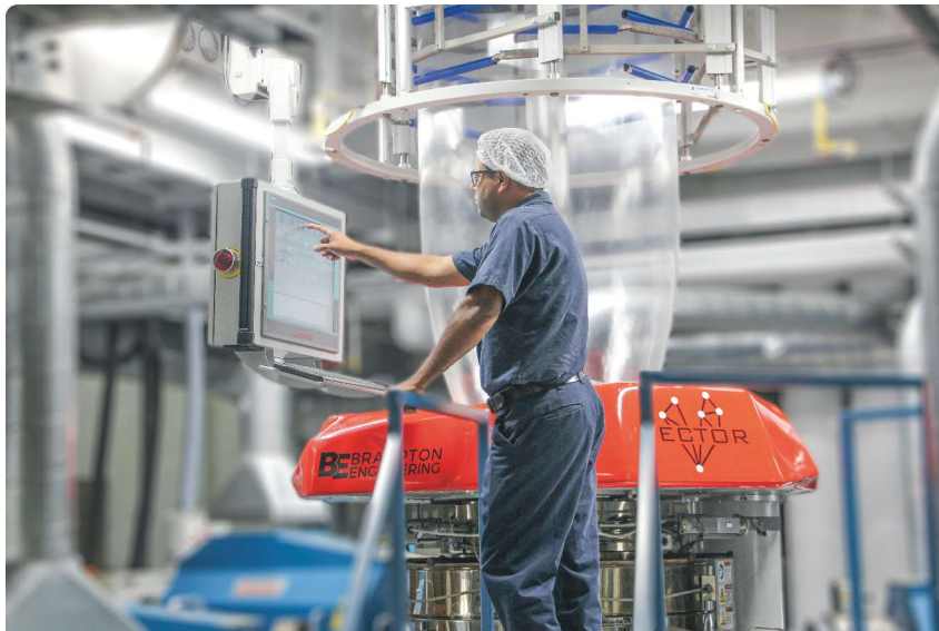
As a result of extremely uniform airflow around the lip, Brampton's Vector S air ring reportedly offers the best startup gauge in the industry by reducing variability by up to 80% compared with conventional air rings.
