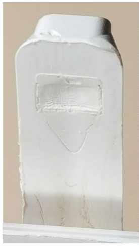
FIG 4 A trapezoidal jump-gate stem with a chisel-type tunnel gate.
