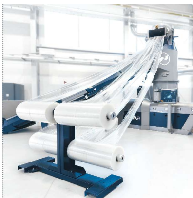
Clean LDPE film waste will be processed live at the Erema booth on an Intarema 1108 T to make high-grade scrap.
