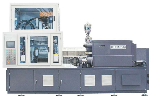
Pet All Manufacturing is exhibiting for the first time its new ISBM-180E all-electric, four-station rotary one-stage PET stretch-blow machine with a 15-ton clamp and six to 10 cavities for containers from 10 to 100 ml.
