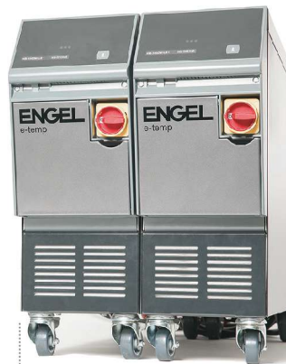
Engel's iQ flow control software networks the new e-temp TCU with energy-saving variable-speed pump together with electronic flow-control valving and the molding machine controller for optimal cooling flow.
