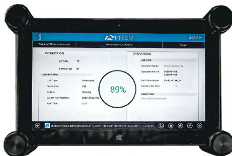
Smart Attend has been integrated with Axiom’s home-grown ERP system, called Prism. Smart Attend screen on Prism tablet shows OEE figure of 89%.
