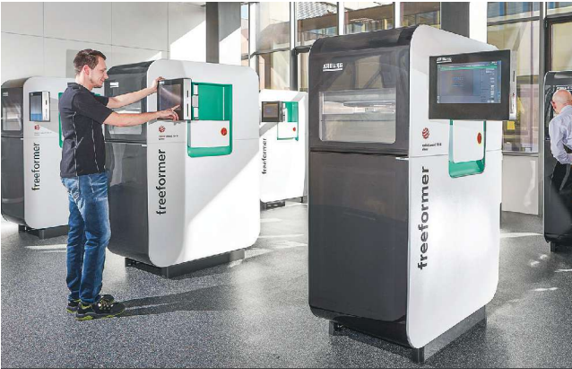
Arburg's freeformer is designed for industrial additive manufacturing of functional parts using standard injection molding pellets. Arburg will also give a presentation on this at the 3D Printing Workshop.
