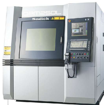
Plustech's OPM250 metal 3D printer combines laser sintering of metal powder and high-speed milling in the same machine. It can make mold components with conformal cooling built in.
