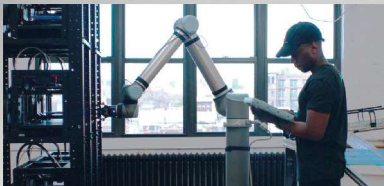
When placed on a mobile base, one UR10 robot can tend one hundred 3D printers.
