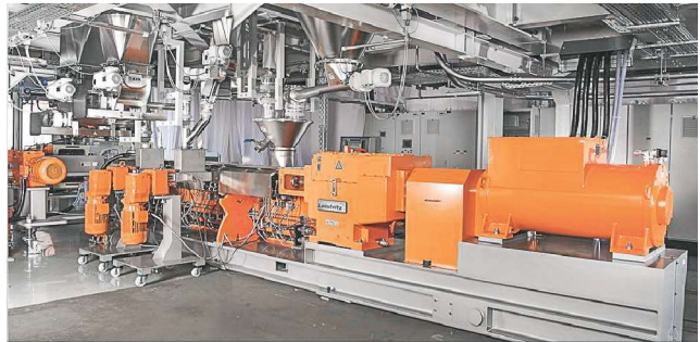
Leistritz is displaying a ZSE 50 MAXX twin-screw that includes a modular design for barrels and screws and insulated barrel covers. The machine will be furnished with two LSB XX series side stuffers.
