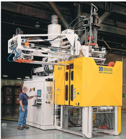
Mini Hercules from Graham Engineering is a new small-shot (2.5 to 8 lb) accumulator-head machine that can perform color or material changes in 1 hr.
