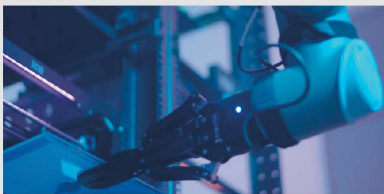
Seamless integration of gripper and robot arm through plug & play UR+ platform.
