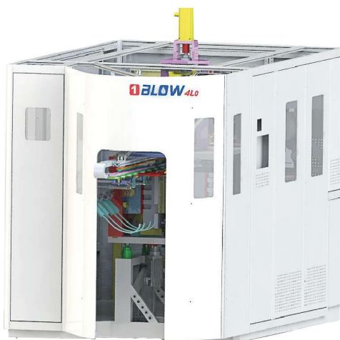
New 4LO all-electric reheat stretch-blow system from 1Blow of France is optimized for custom PET bottles with complex shapes.
