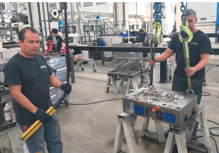
The middle of Integrity's three bays is dedicated to mold assembly with 22 separate work cells.
