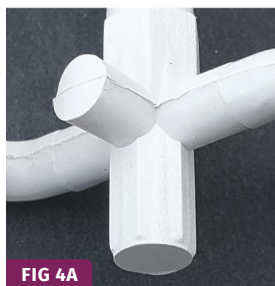
RTO with a hex EDM'd for a full-round runner (left) and a trapezoidal runner (right).
