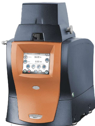
Dynamic mechanical analysis (DMA) has been proposed as a more valid alternative to HDT for at least 20 years. Today's more critical engineering applications for plastics make a change all the more urgent. (Photo: DMA 850 from TA Instruments)
