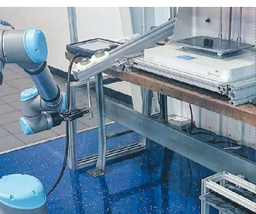
EVCO is applying UR cobots to tasks from insert loading, assembly and packaging to tending its 3D printers, as in this test cell.
