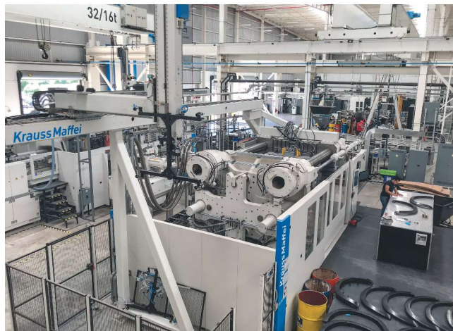
Integrity offers its customers five injection molding machines, ranging in clamp tonnage from 320 to 2300 tons. Show here is a 2300-ton KraussMaffei machine.
