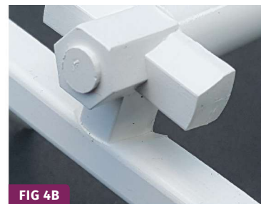
RTO with a hex EDM'd for a full-round runner (left) and a trapezoidal runner (right).
