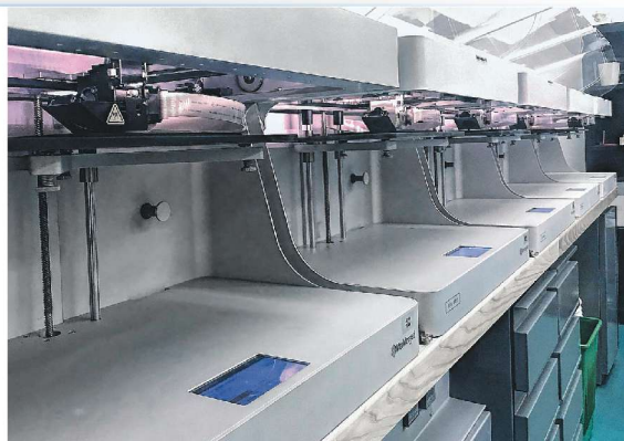
A “printer farm” with a dozen Markforged 3D printers for prototypes and short runs of up to 600 parts is a new compliment to EVCO’s injection molding business.
