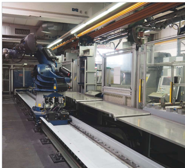
Four EDM machines from OPS Ingersoll are connected via a robot. Hofmann started its first automation efforts in its EDM department. Because electrode milling and EDM are time-consuming processes, they are ideally suited for automation.
