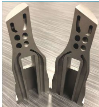
Krieger Craftsmen offers additive manufacturing of mold components, like this core printed in H13 that is split open to show its balanced internal cooling channels.
