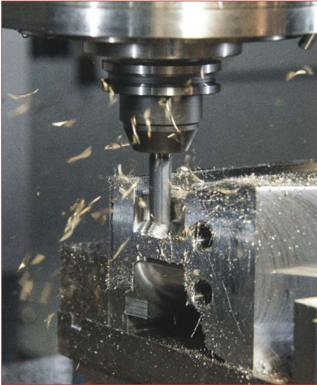
Dynamic motion machining is a significant timesaver for shops that want to rough molds as quickly as possible.
