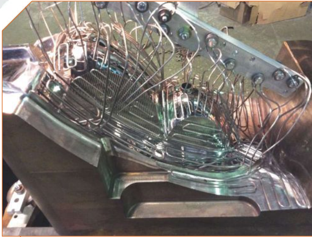
Shown here is a lighting mold refurbishment utilizing conforming wire anodes for the mold body. This helps to achieve a consistent plating thickness over the highly complex surface geometry of the mold for more even wear and excellent release characteristics.
