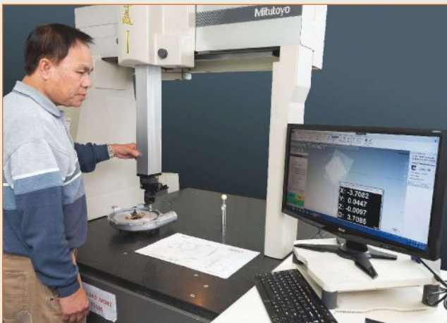
Hyatt Die Cast uses Verisurf Software to verify first article die castings against a paper drawing, as shown here. Verisurf also works with all CAD files, including 2D and 3D CAD models. The operator can then complete detailed first article inspection reports in the software program.
