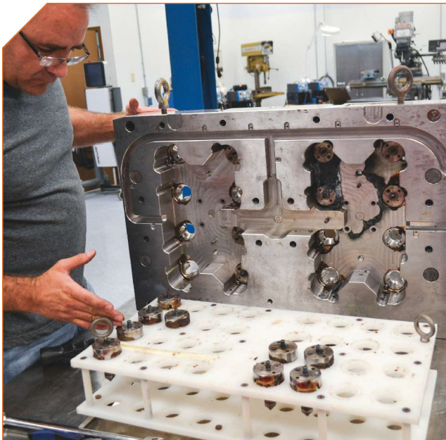
Nozzles should be removed carefully instead of being thrown in a basket for cleaning.
