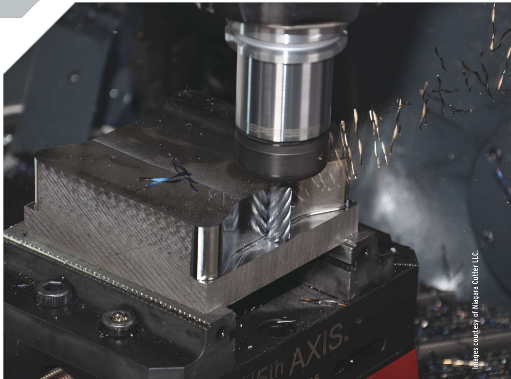
This solid carbide cutter side mills 4140 with an optimized roughing strategy.
