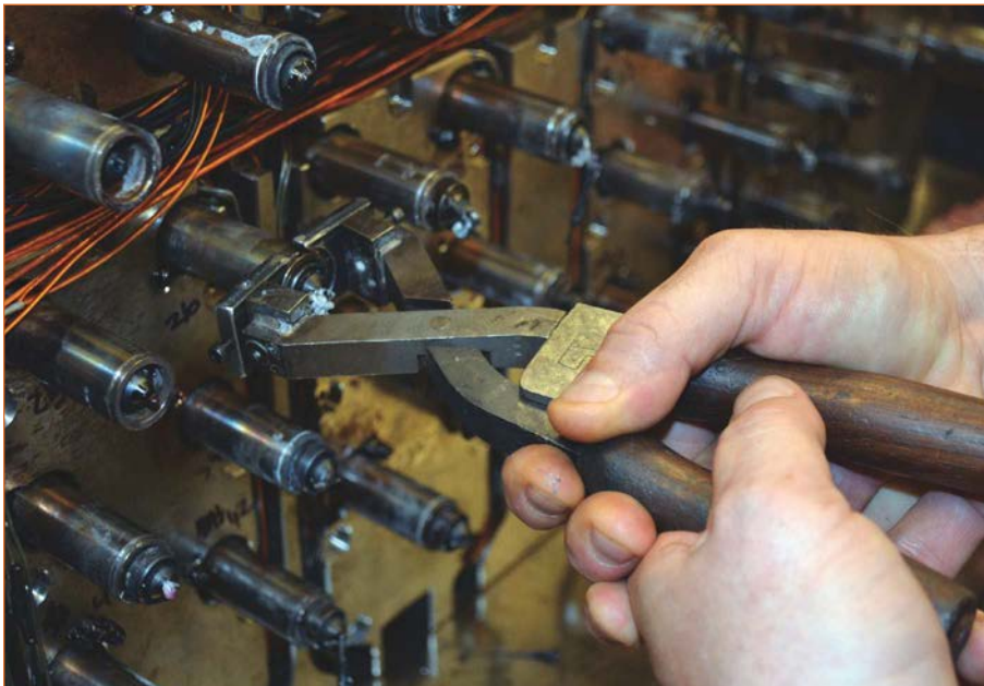
This special tool provides technicians with a firm grip when they are removing stubborn heaters. The tool will not damage the outer sheath.
