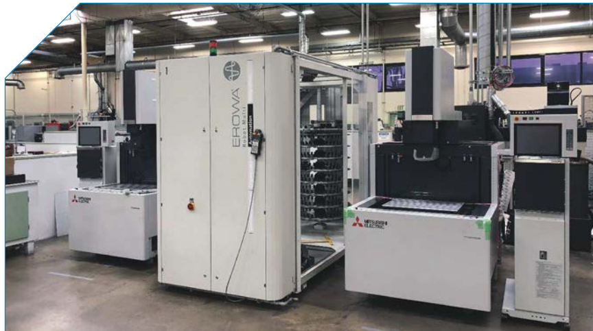
This Mitsubishi sinker EDM cell is integrated with an Erowa Robot Multi. It is one of several equipment purchases that will help Fairway Injection Molds expand its capabilities and grow as part of the Westfall Technik group of companies.
