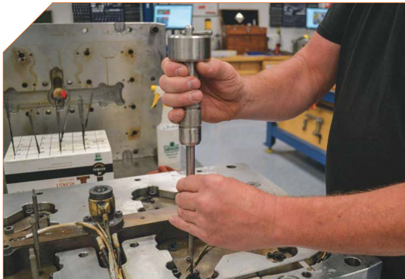
Here, a technician uses specifically weighted slide hammers to control the force he is applying as he removes valve pins. This technique reduces the risk of damage.
