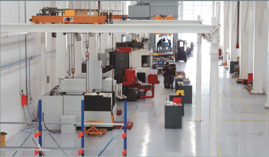
Siebenwurst invested in both three-axis and five-axis milling machines from DMG MORI, a 500-ton Williams & White die-spotting press, a mobile laser-welding machine, indoor and gantry cranes, a wire EDM machine from Mitsubishi, a die-sinking machine from ONA and the installation of a CAD/CAM workstation from Tebis.
