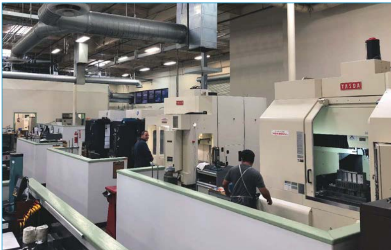
Employees at Fairway Injection Molds run Yasda CNC machining centers in the company's hard-milling department. Fairway recently took delivery of a new Yasda YBM950V hard-machining center (pictured on the far right) to expand its ability to supply customers with very precisely machined parts, like shut-offs and other mold components, without the need for secondary handwork.
