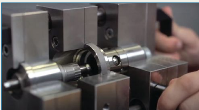
Round latch locking unit for precise opening of a second mold parting line in injection molds.
