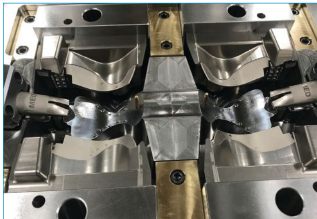
This medical device two-cavity mold features multiple compound actions.
