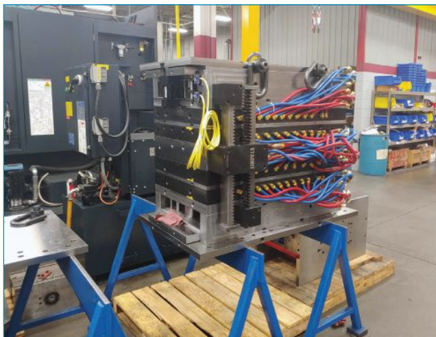
This stack mold design allows greater cavitation within a smaller press platen size.
