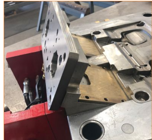
With a laser-sintered 420 SS cooling plate mounted to a mold, the mold can run at +300°F degrees while keeping the cylinders cool and eliminating issues with the limit switches.
