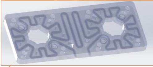
This laser-sintered 420 SS cooling plate with integrated circuits between mounting holes covers the entire mounting surface with even temperature control.
