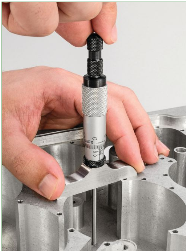
Electronic and mechanical depth micrometers measure parts with depth features like internal notches in 1 to 0.0001-inch increments accuracy and 50 millionths (0.00005-inch) resolution.
