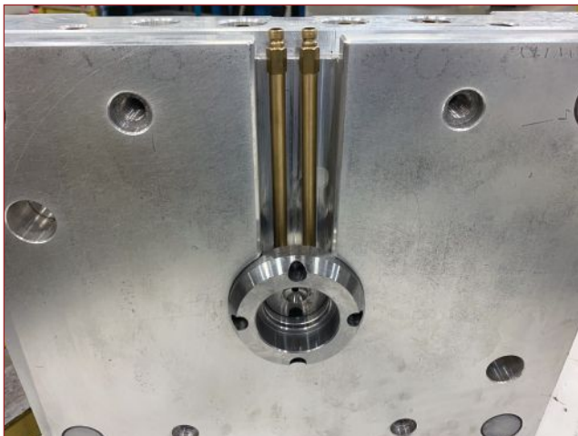
Cavity side of mold showing how water lines were plumbed into conformally cooled sprue bushing.
