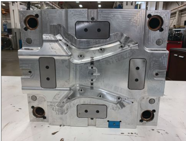
Core (B) side of a TPV spoiler seal tool showing placement location for the four PA 6/6 fasteners (left) and B-side of part showing fasteners attached (right).
