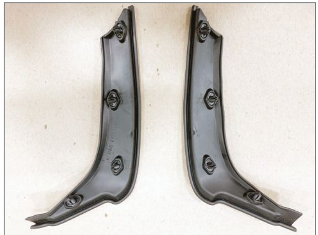
Core (B) side of a TPV spoiler seal tool showing placement location for the four PA 6/6 fasteners (left) and B-side of part showing fasteners attached (right).
