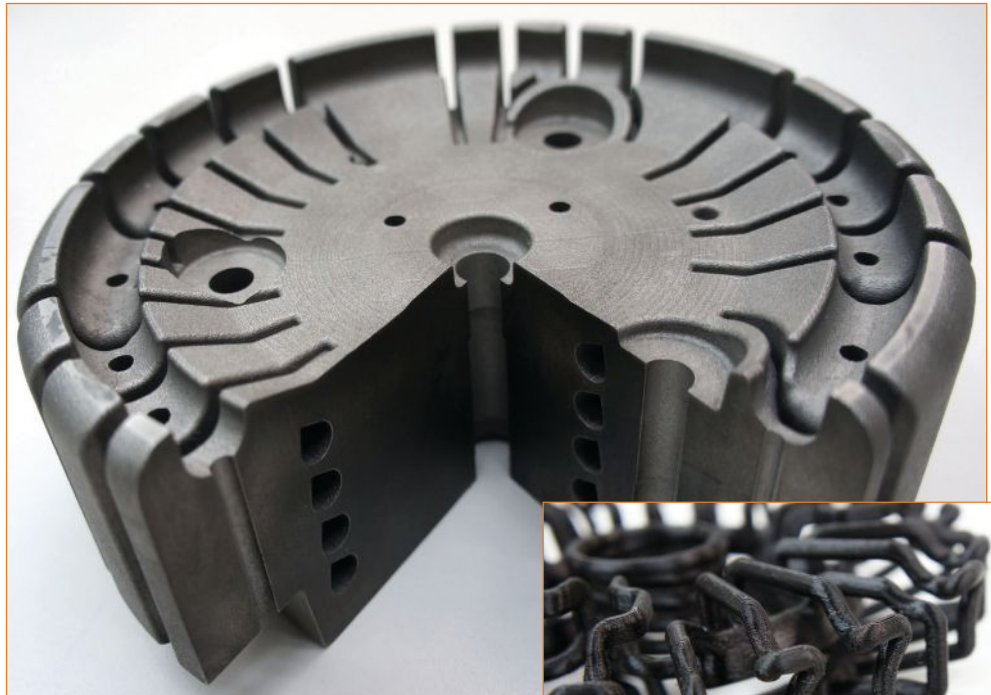
The 3D-printed metal insert in the first picture (which still needs finishing) is cooled by a serpentine network of water channels represented by this 3D-printed plastic model. The cutaway from the demo part above also reveals easy-to-print teardrop-shaped channels.
