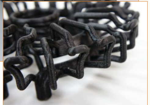
The 3D-printed metal insert in the first picture (which still needs finishing) is cooled by a serpentine network of water channels represented by this 3D-printed plastic model. The cutaway from the demo part above also reveals easy-to-print teardrop-shaped channels.
