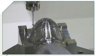
During machining of this mask frame mold cavity, a probe can automatically realign the cutting tool and update offsets in reaction to changes in temperature.
