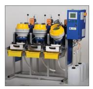
els come with a mobile frame, ideal for cellular and JIT production. A wide variety of additional features are also available including integrated ultrasonic cleaners, on board media storage, a direct compound feed system and parts separation options.
