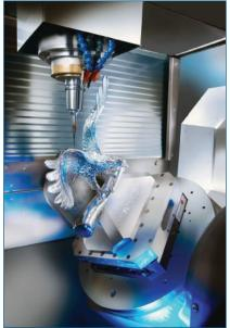
OPS Ingersoll's Eagle five-axis hard-milling machines are designed to mill both graphite as well as hardened steel quickly and efficiently. These bridge-style machines are very stiff, stable, and accurate so the mills can run at high rpms. A composite/concrete base provides high damping. The systems also use twin ball screws in the X and Y axes for high-speed acceleration/deceleration and provides high thermal compensation in all axes.
