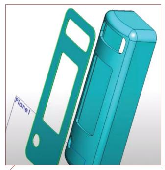
The area of a movable core is the area exposed to plastic projected along the core axis onto a perpendicular plane. Information on how to use CAD systems to calculate the projected area is available online-see a video example from SOLIDWORKS-Surface Area Projection YouTube Go Engineer, which demonstrates selecting surfaces and projecting onto a plane.
