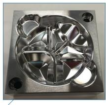
To determine which machinery OEM had the best milling center, Cavalier modified an earlier design developed by Okuma Corp. (Oguchi, Japan) and set up a test-cut competition for machine makers called the "angry monkey." The clear winner of the test was OPS Ingersoll, which was 30% faster than some other competitors. to gap conditions, lowering energy usage and electrode wear, and cutting graphite costs dramatically. We knew that would be a game-changer for North American moldmakers."
