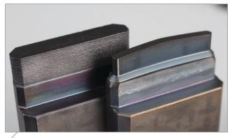
The top of this hybrid stamping die is 3D printed using Kolibri's custom SLM machines, made from Colima, a wear-resistant steel with a high carbide content and additional toughness.
