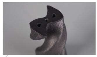
This 3D-printed end mill is made from Kolibri's Cotopaxi steel with 65 HRC and added carbides for additional hardness and wear-resistance. Cooling channels can be easily integrated and the cutter is ready to use as it comes out of the SLM machine, only the cutting edges need to be finished.
