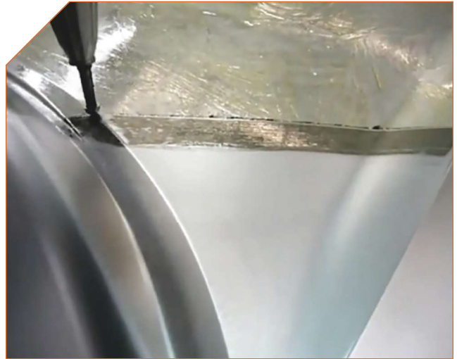
Machine-hammer peening is applied through the operation of a controllable electro-magnetic hammer head imparting rapid reciprocal motion of a striker ball against a workpiece surface. This image demonstrates the before and after of a mold surface being peened.
