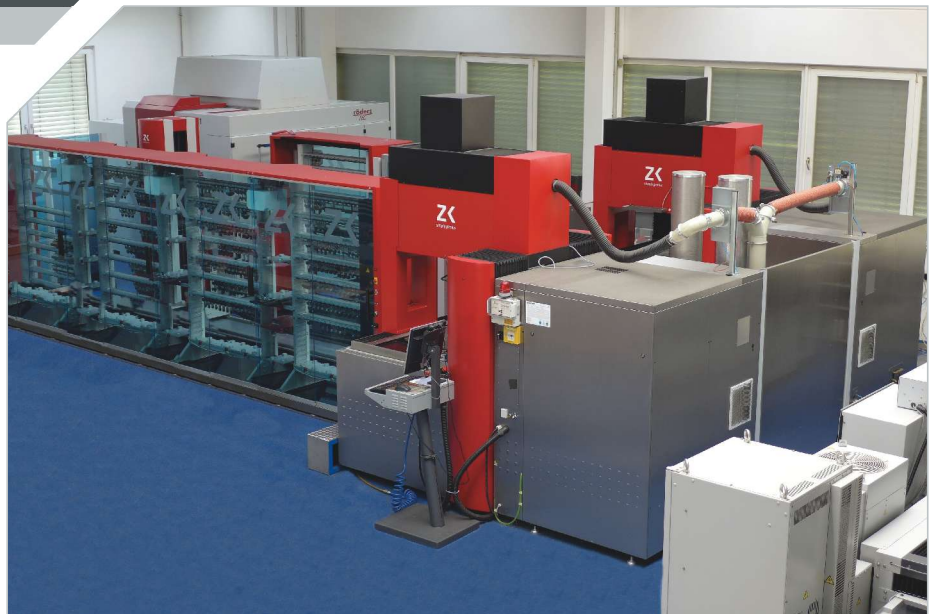
W. Fassnacht Werkzeug- und Formenbau has continuously invested in automation, including a five-axis machining center, CNC measuring machine, two EDM machines and a handling system.
