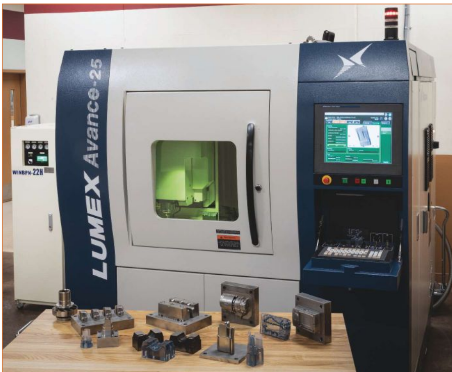
Custom Mold & Design's LUMEX Avance-25 hybrid machine from Matsuura Machinery can tackle complex geometries and conformal cooling as shown by this display of part samples.
