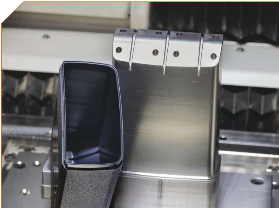
Custom Mold & Design is building a new core insert for this cover to reduce warpage and improve cycle time. Note the curve on the left side of the plastic part that should be straight.
