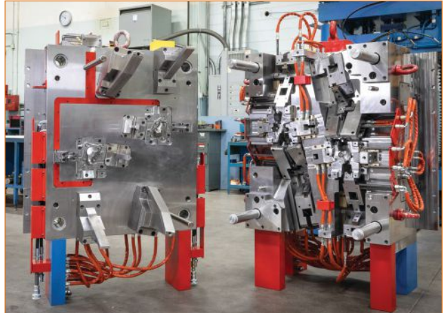
This automotive under-the-hood water outlet mold consists of 420 manufactured parts, 24 of which are moving. The mold has two cavities, each having 12 moving parts (slides, lifters, guides, pins, etc.), making a total of 24 moving parts for a part that's only the size of your fist.
