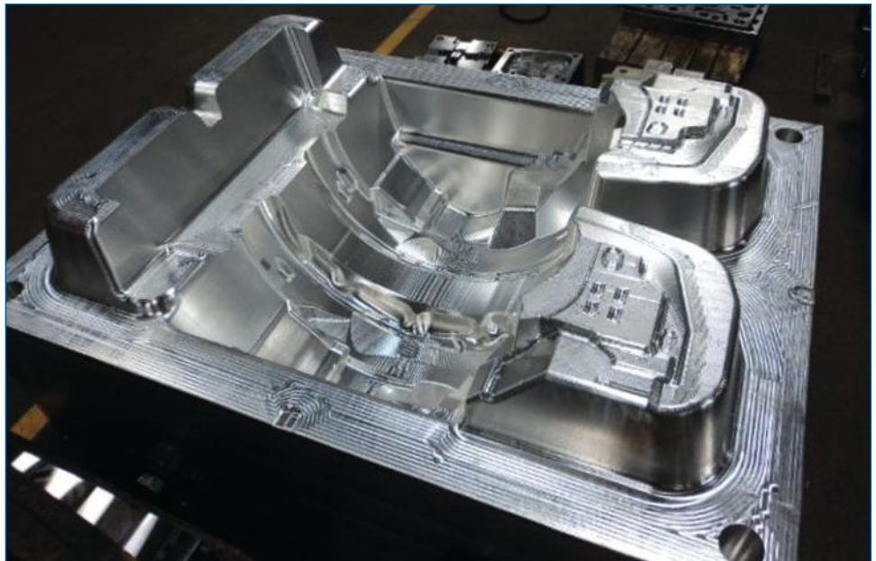
Unique Tool and Gauge produced this high-volume aluminum tool for the front wheel well liner of the 2011 Honda Civic that was produced in the U.S.
