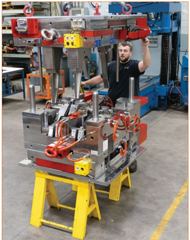
Although everyone in the shop handled some aspect of this mold at one time or another, the core team to take it on was established with one-on-one training based on a two-minds-are-better-than-one attitude. This team worked together with engineering on part design to provide the optimal design for manufacturing (DFM) to keep maintenance costs down and to make the mold more manufacturing-friendly.
