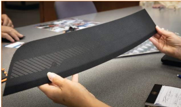
The holes on this automotive defroster vent appear to be round, but each hole actually has five sides, making the manufacturing very complicated. The file size alone is over 2 gigabytes.
