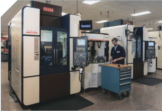
Yasda micromachining centers equipped with robotic part changers perform precision five-axis machining unattended in continuous operations through the weekend.
