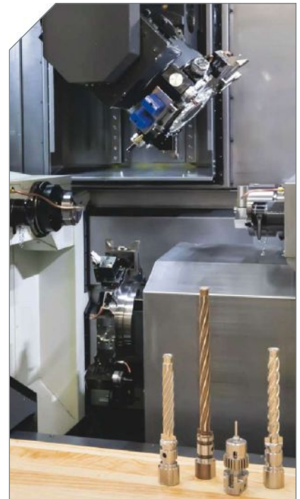
These examples show some of the variety of parts machined complete in one operation from barstock on three Nakamura-Tome multitasking machines that combine turning and milling operations in one machine.
