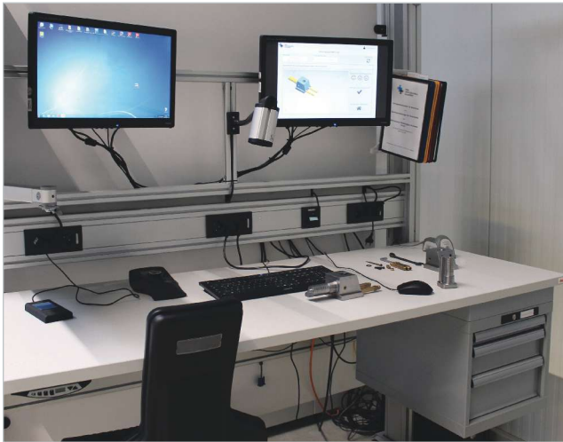
The digital assembly table is supposed to reduce errors and increase efficiency during mold assembly and maintenance through digital images and movies.
