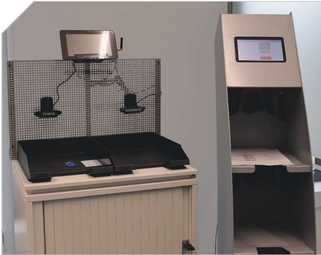
WBA has developed a scanner, which automatically scans all order data when the worker places the order sheet in the appropriate tray. The ultimate goal is a paper-free organization.
