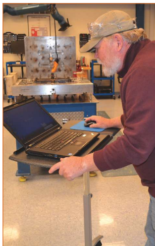
A mobile computer station (left) as opposed to a mobile stand (right) should have a suitable height and weight for stability, shelving for additional equipment and large, soft, lockable rubber wheels to ease movement around the shop.
