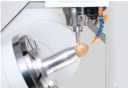
Egg Machining Shape-followed Machining Even Cutting Depth
