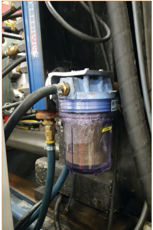
Filtering individual circuits as close to the mold as possible removes major solids from the cooling source and prevents them from collecting in areas close to the heat source inside the mold insert where calcium builds up.
