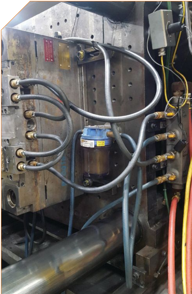
Place a local filter as close to the mold as possible whether you are running off a central process cooling system or a local thermolator at the press.
