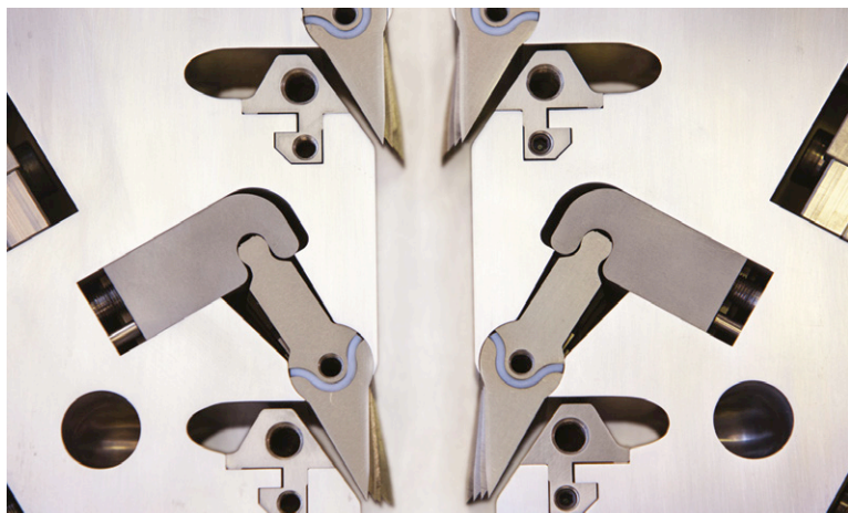
Above: Reicofeed-Pro adjusts the thickness of multi-layer films on the fly to cut material costs
