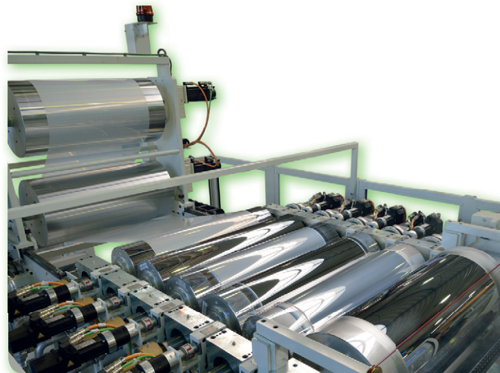
Close-up of Multi-Touch roll stack from above
