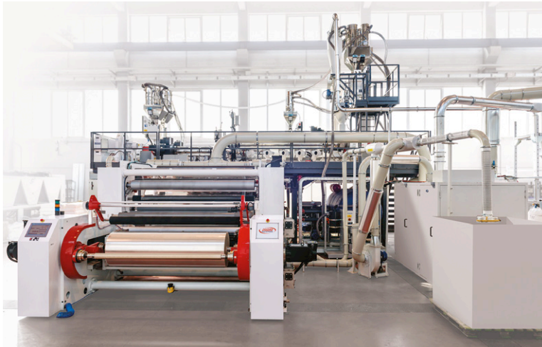
Above: Amut has developed a new line for the production of cast PP film
