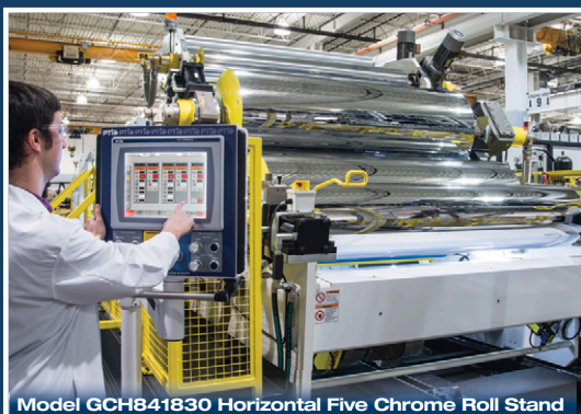
Model GCH841830 Horizontal Five Chrome Roll Stand
