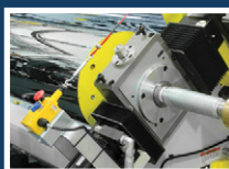
US Pat. #9,182,067 Chrome Roll Skew Mechanism
