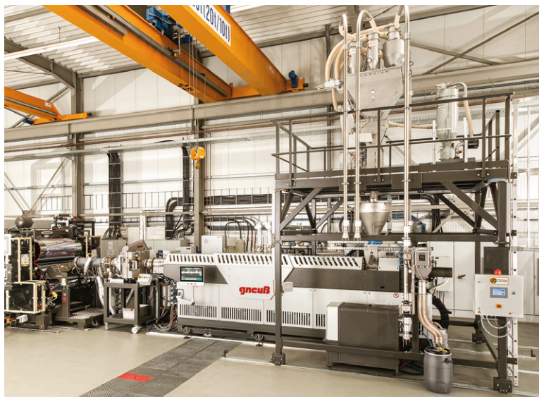
Above: The Gneuss Processing Unit (GPU) has been successfully used in PET sheet extrusion
