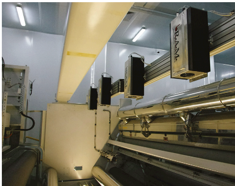
Above: NDC's new Web Surface Inspection Systems help manufacturers to achieve zero defects
