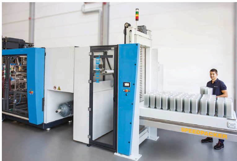
Above: Kiefel's SpeedPacker is a buffering and unloading station that is fully integrated into steel rule cutting machines, including those from other manufacturers
