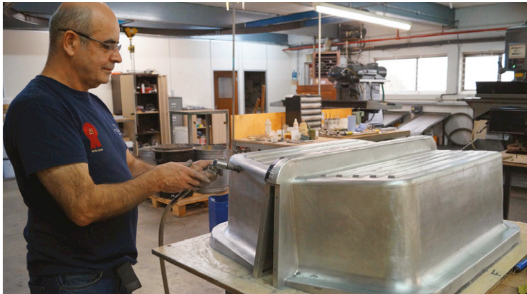
Above: Tony Harris, a pattern maker at Belgrade, puts the finishing touches on an aluminium mould to make ABS wheel boxes
