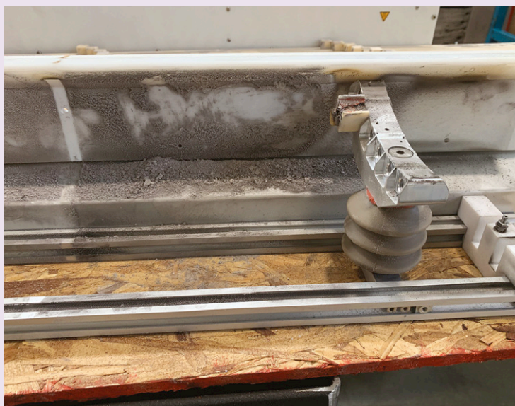
Above: Cleaning electrodes regularly is vital in order to surface treatment equipment working at maximum output, says Vetaphone
