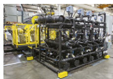
5 Zone Temp Station
