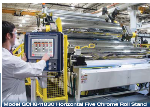
Model GCH841830 Horizontal Five Chrome Roll Stand
