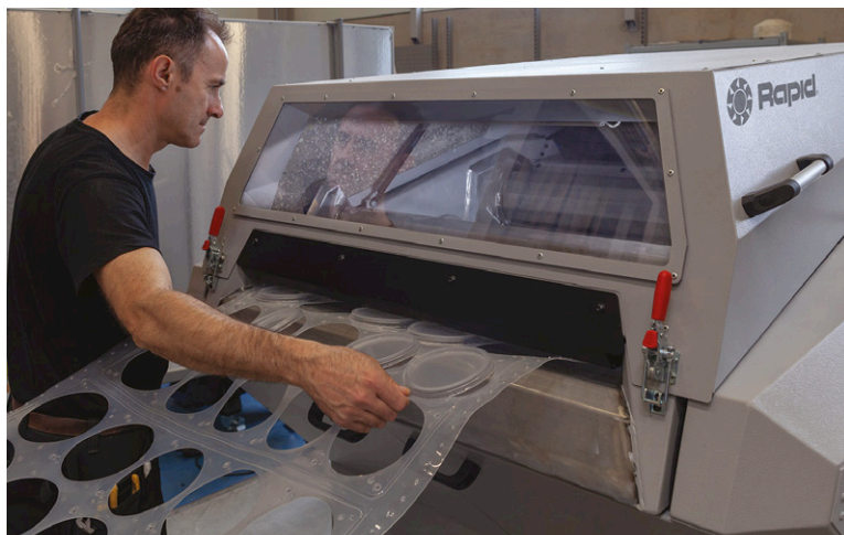
Below: Rapid's ThermoPro granulators are designed for in-line processing of skeletal waste
