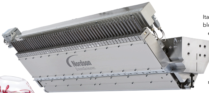
Above and left: An automatic die helped Innovia improve tolerances and reduce start-up times in shrink film production for soft drink bottles
