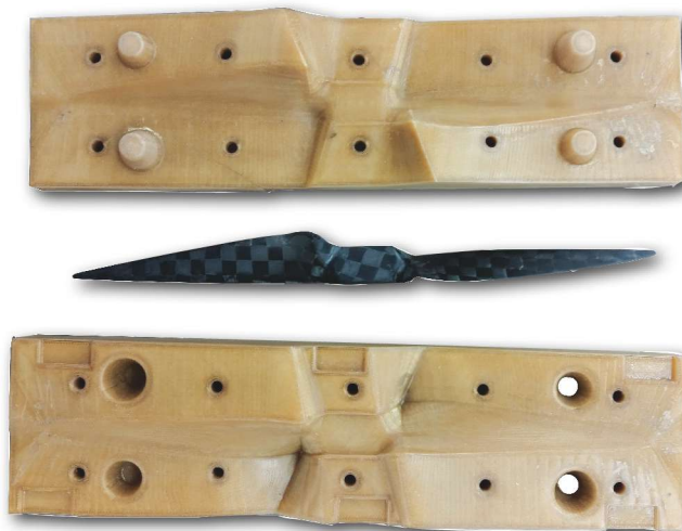
FIG. 6 Additive manufacturing tooling alternative
