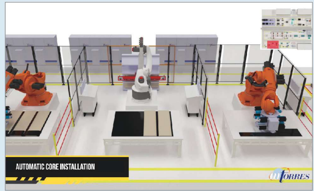
4 On a parallel production line, the flat floor panels are produced. A moving line brings flat table molds into position in front of stationary robots, which lay the lower skin, core panels and upper skin, in sequence.
