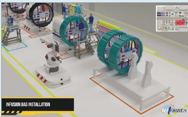
3 After completion of the ring layup, the positioning robots move the rings to the bagging area, where the rings are prepped for resin infusion, and cure. Note that the flat plates that extend across the bottom of each ring will act as supports for the fuselage cabin's floor panels.
