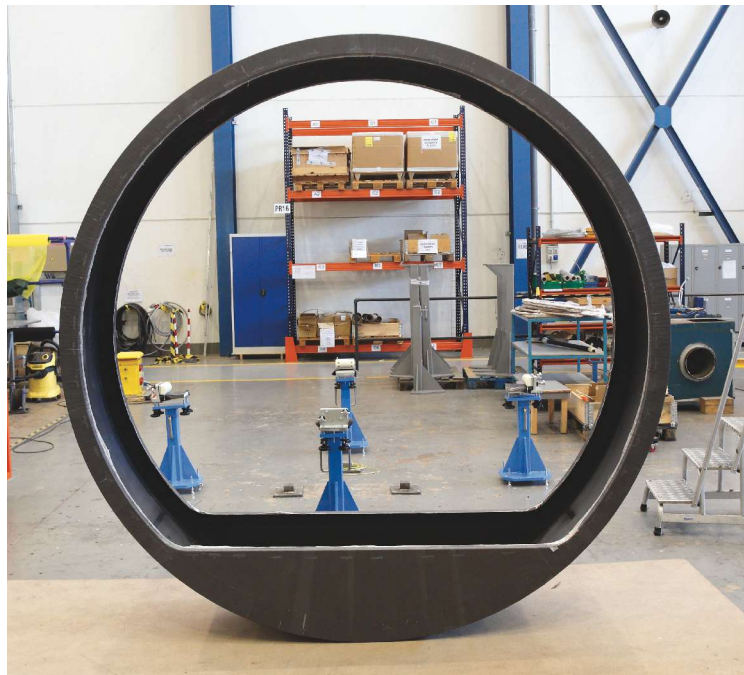
FIG. 1 Replacing tools and stringers with ride-along rings
