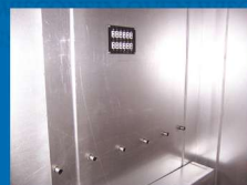
Interior Thermocouple Jack Panel & Vacuum Stubs
