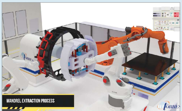
6 After oven cure is complete, parts are transported to the machining area, where a robot trims and creates openings in the rings' floor supports, and trims the floor panels. Shown here is a robot collapsing and removing a ring's mandrel. Following this step, the elemental parts undergo non-destructive inspection.
