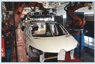
The pre-assembled sunshade module with glass roof is positioned by robot onto the vehicle and then bonded to the vehicle roof.
