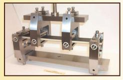
Reversed Cycle Flexural Fatigue
