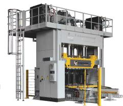
and thermoplastics like PPS, PEI, PEEK or similar. Press features include maintenance-free cylinder technology, servo/hydraulics with pressure accuracy of ±1%, optimized pump technology, active parallel control, platen heating up to 500°C, automation and robot integration, flexible software, data management and Industry 4.0 compatibility. Booth J23.
