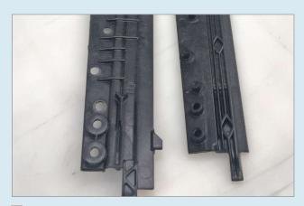
3 Final moldings of top and bottom sides of one pair of rails prior to ultrasonic welding.
