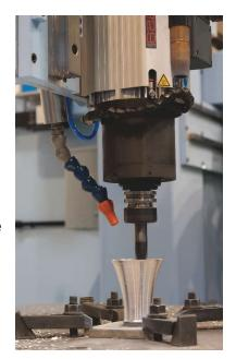
envelope that is 2 by 2 by 2 ft. The machines use a dual carriage, which includes an additive deposition head and a 3-axis, 12-HP, 24,000-rpm spindle. Booth S29.
