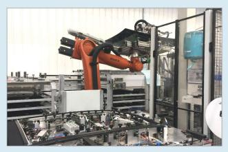
After dispensing adhesive, robot prepares to bond glass to top of sunroof system.
