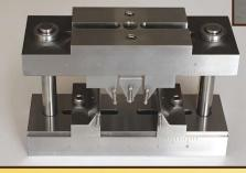
Three and Four Point Short Beam Fixture ASTM D 790, D 6272, D 7264, D 2344
