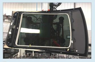
8 Fully assembled and pretested module ready to install on vehicle. The sunroof's water seal is carried on the glass and is achieved using the PUR adhesive that joins the glass to the rest of the module.
