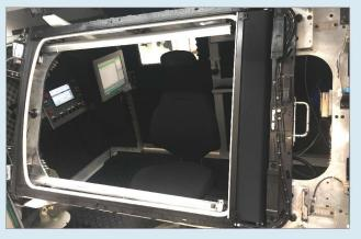
6 Final preparations for roller-blind module prior to glass bonding.
