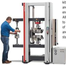
kits for fiber composite materials and compression test kits for end loading. The company's AllroundLine system is said to to perform more than 20 types of composites tests in compliance with more than 100 test standards. The TestXpert III test
