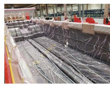
FIG. 2 Infusion of bus body, upper and lower
