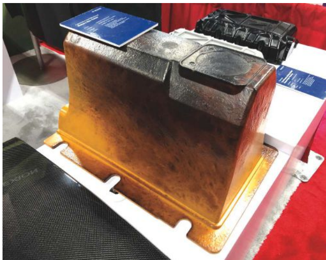
■ This flame-retardant battery box cover constructed of phenolic SMC from Hexion retains 60-70% of its material properties after aggressive fire testing.
