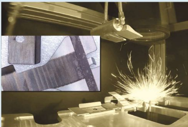
3 Inside the structuring cell, a high-power fiber laser creates undercuts in the surface of the bracket to be joined to the composite roof stiffener.
