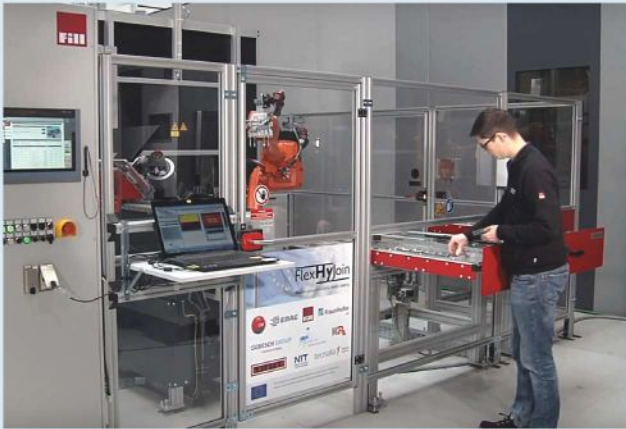
1 TPC roof bows and metal brackets are manually loaded into the parts drawer of the FlexHyJoin cell. The drawer is closed and production begins. Source, all steps | FlexHyJoin
