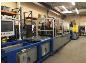
Interactive Touchscreen PLC Controls the machine operation
