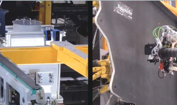
2 Before ribs are bonded to the shell, each is scanned with a laser measurement device as is the area of the shell where it is to be mated.
