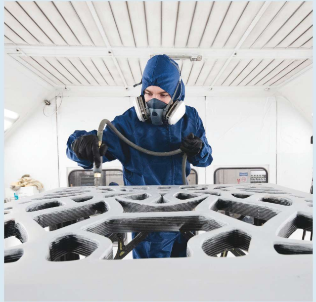
3 The external surface of the cab is sprayed with the self-leveling filler/coating, which is formulated to hide the print lines and to chemically bond to the carbon fiber-reinforced ABS substrate to provide a paintable surface.
