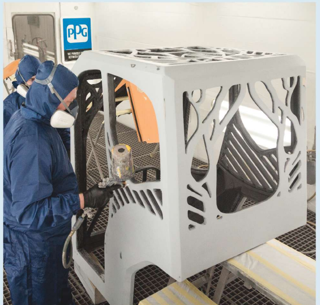
4 After the self-leveling filler dries, its surface and edges are sanded to provide a smooth, paintable surface. Then a primer (shown here) is applied to the coated, external surface of the cab.
