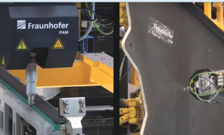
3 Rib and shell surfaces to be bonded are treated with atmospheric plasma to increase surface energy activation for higher-strength adhesive bonds.
