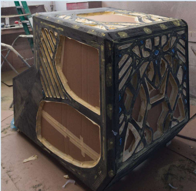
2 After printing, the parts are assembled with a combination of snap-fit joints, screws and adhesive. After assembly, the cab is masked, as shown here, to ensure that a patent-pending, self-leveling filler/coating is applied only to the external, paintable surfaces.
