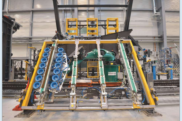
5 Robot with flexible gripper system (blue vacuum cups) removes CFRP rib (mounted in aluminum fixture) from universal frame which can hold all 8 ribs needed for each VTP shell.
