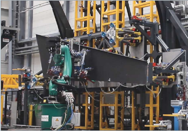
1 A composite VTP NG shell section is robotically placed into a flexible, automated holding fixture within the rib-shell assembly area.
